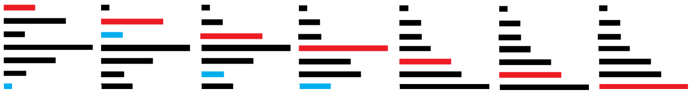
Figure 1. Selection Sort - Red represents the current starting position. Blue represents the smallest so far by end of pass (except where start is also smallest, then it is just shown in red). Only the state of the elements right before the swap (see code below) are depicted in this picture.
